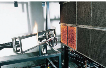
A3) The panel is 50% charred.
