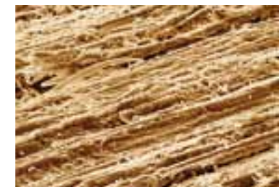
Wooden surface after sanding with silicon carbide.
