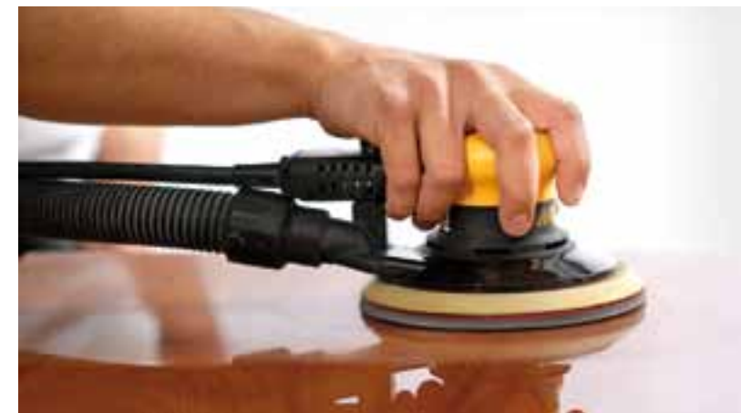
Sanding of top coat before polishing.
