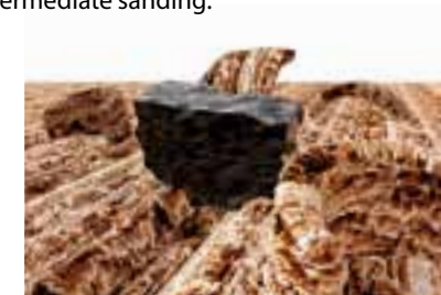
Silicon carbide grains cut through hard wood.
