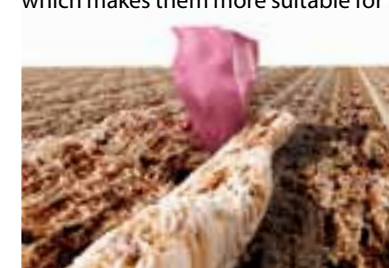
Aluminium oxide grains plough into soft wood types.
