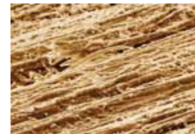
Wooden surface after sanding with aluminium oxide.
